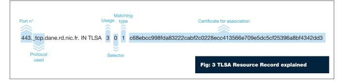
As shown in Figure 3, the TLSA resource record consists of four fields: the "certificate Usage", "a Selector", "a Matching type" and the "Certificate for association" data. The application must match the 'certificate for association data field' in the TLSA RR with the target certificate (i.e. the certificate obtained from the domain's web server) based on the other values (certificate usage, selector and matching type) in the TLSA resource record.
