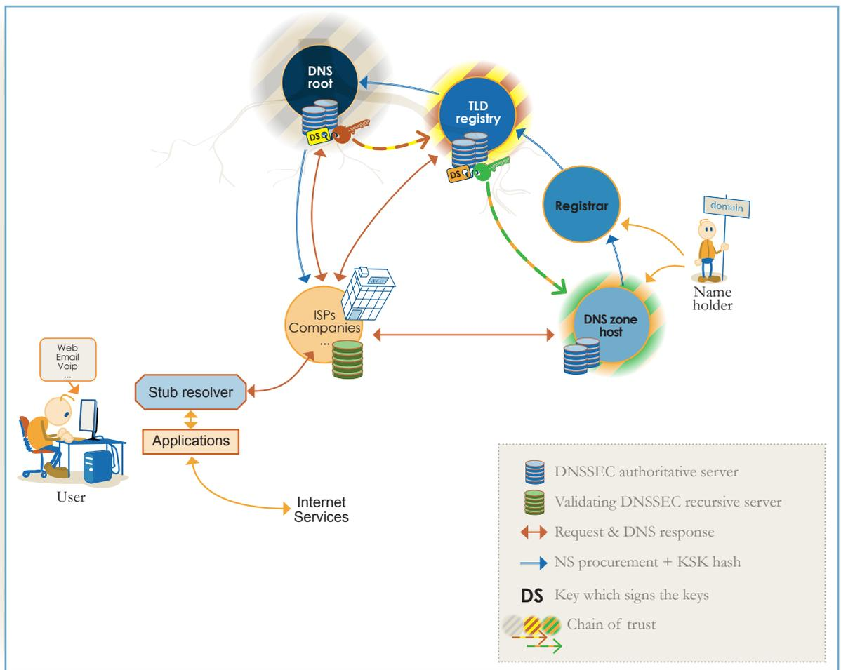
Components of the DNSSEC chain of trust
