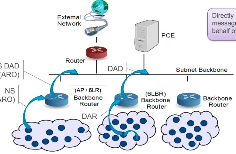
Directly upon NS(ARO) or indirectly upon DA message, the backbone router performs DAD behalf of the wireless device.
