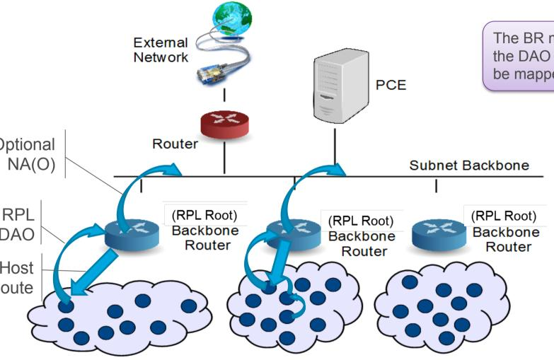
The BR maintains a route to the WSN node for the DAO Lifetime over instance VRF. VFR ma be mapped onto a VLAN on the backbone.
