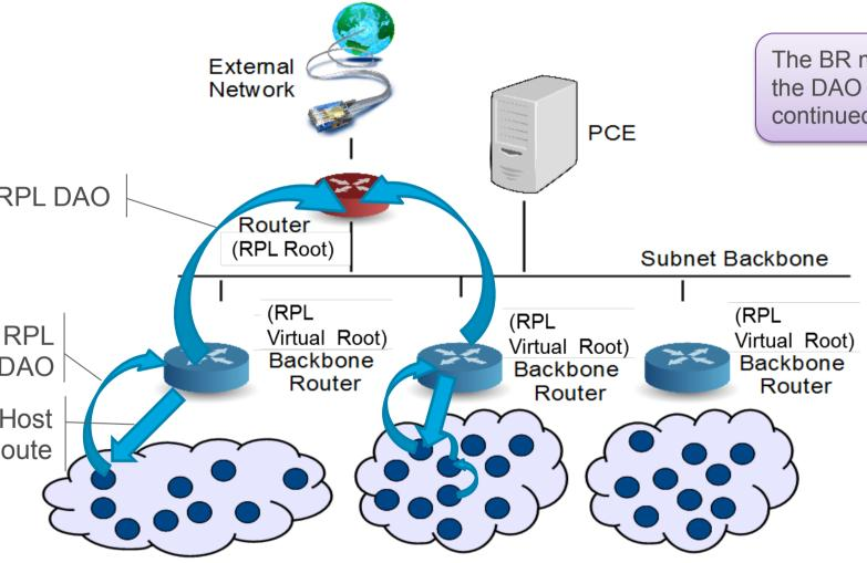
The BR maintains a route to the WSN node for the DAO Lifetime over instance VRF that is continued with RPL over backbone.
