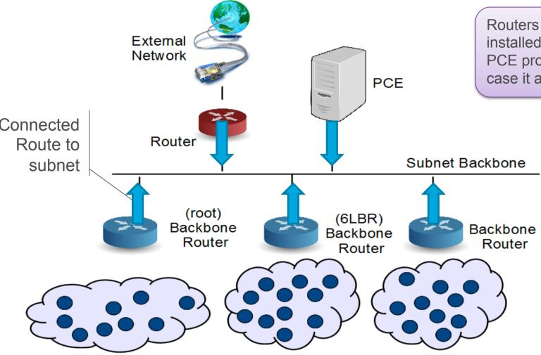
Routers within subnet have a connected route installed over the subnet backbone.
